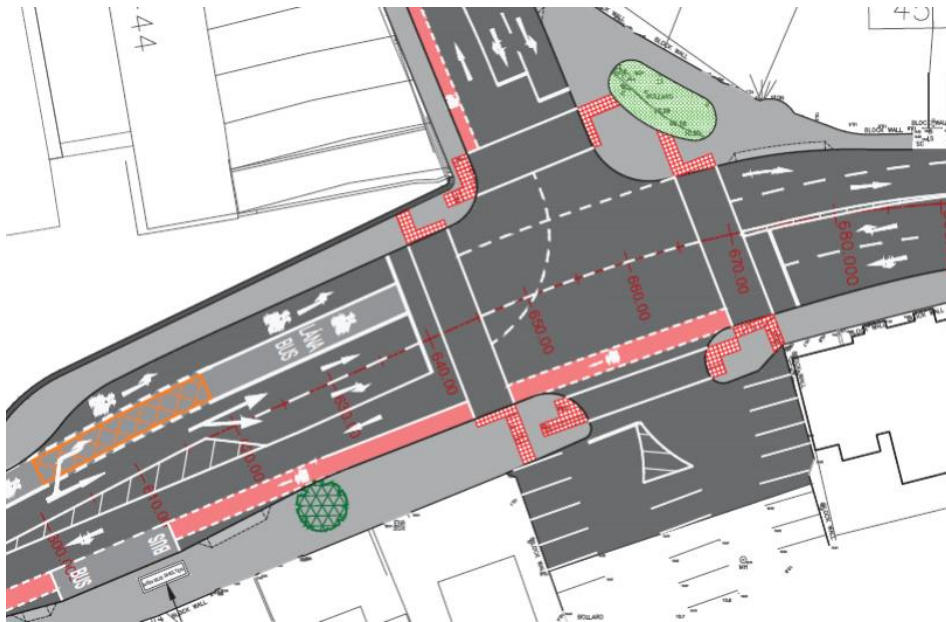
Figure 3 Skehard Road/Church Road Proposed Junction Upgrade Layout
